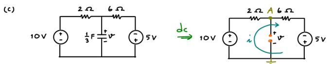
Method 1: Mesh analysis: There is only one mesh. Applying KVL gives  $10 - i \times 2 - i \times 6 + 5 = 0$ . This implies i = 15 A. So,  $v = 10 - \frac{15}{8} \times 2$ Method 2: Nodal analysis: KCL @ A gives = 25 = 6.25 V
